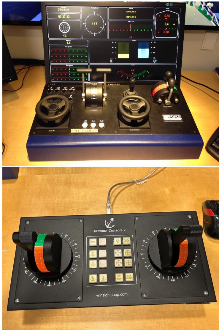
Figure 4-2 Ship main control hardware console. Top console for regular engines and bottom console for azipods (used for Workshop No. 2).
